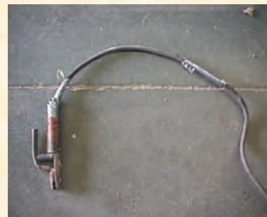
This welding lead has 2 problems with it. It has repairs within 10 feet of the electrode holder and the repairs have been made with duct tape.
