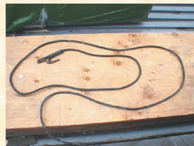
Welding leads are required by OSHA to be free from repairs within 10 feet of the stinger.
